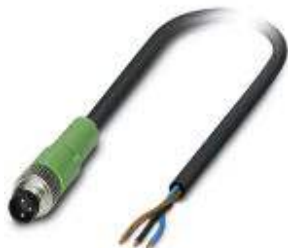
Sensor/Actuator cable, 3-position, PVC, Black RAL 9005, Plug straight M8, on Free cable end, Cable length: 10 m
