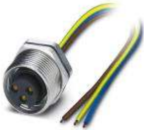
Sensor/actuator flush-type socket, 3-pos., 7/8", rear mounting with M26 fastening thread, with 1.0 m PE litz wire, 3 x 0.75 mm 2
