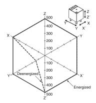
The value at which malfunction occurred was measured after applying shock to the test piece 3 times each in 6 directions along 3 axes.
