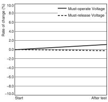
Characteristics were measured after applying vibration at a frequency of 5 to 200 to 5 Hz, acceleration of 44.1 m/s<sup>2</sup> to the test piece (not energized) for 2 hours each in 3 directions. The percentage rate of change is the average value for all of the samples. Note: The Upper limit of double amplitude: 10 mm P-P
