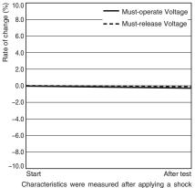
Characteristics were measured after applying a shock of 490 m/s<sup>2</sup> to the test piece 3 times each in 6 directions along 3 axes. The percentage rate of change is the average value for all of the samples.
