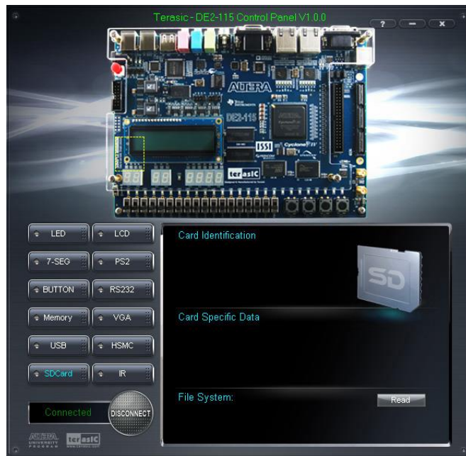
Figure 3-10 Reading the SD Card Identification and Specification
