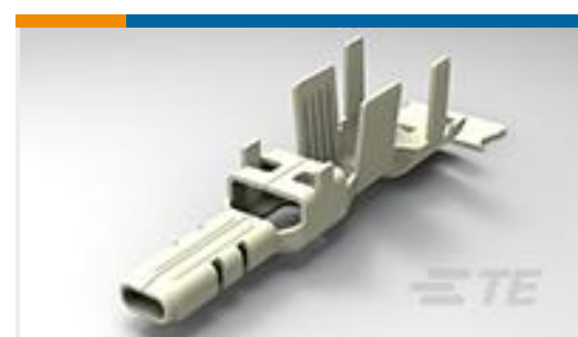
TE Part #63963-1 250 FASTON FLAG REC 18-14 AWG NPST
