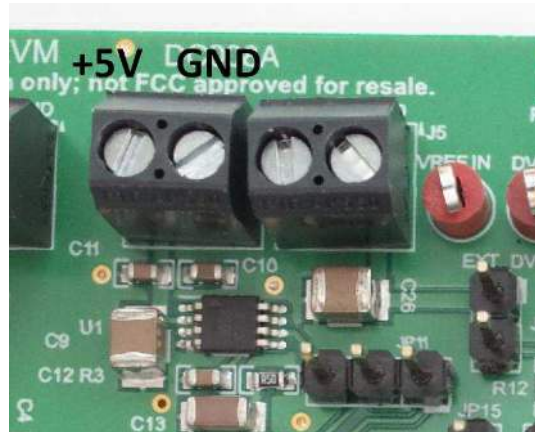
Figure 5. Onboard Reference Supply Connections
