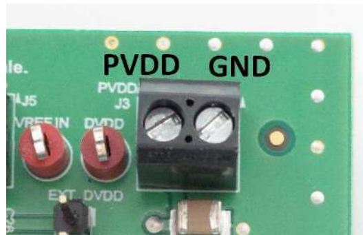
Figure 3. PVDD/AVDD, and DVDD Supply Connections
