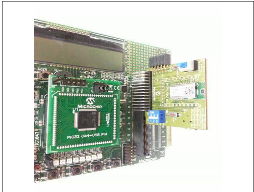
FIGURE 1-3: BM78 EVB BOARD INSERTED INTO PICtail™ INTERFACE
