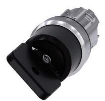
Key-operated switch O.M.R, 22 mm, round, metal, shiny, lock number 73034, black, with 2 keys, 2 switch positions O<I, momentary contact type, Actuating angle 45°, 10:30h/12h, key removal O, with laser labeling, lower case
