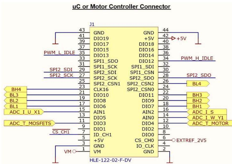
Figure 1: 44 pin Motor Controller Connector
