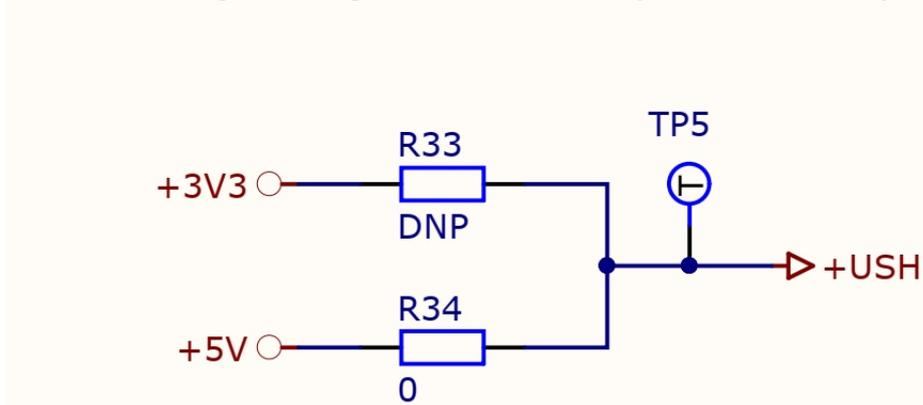
Figure 2: Power supply select for shunt amplifiers
