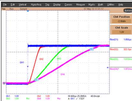
Figure 25. +Power up with different slew rate settings
