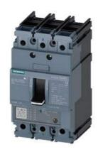
circuit breaker 3VA5 UL frame 125 3-pole, starter protection TM120M, AM, In=30A without overload protection short-circuit protection li=3...7 x In nut keeper kit on both sides
