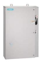
Non-reversing motor starter, Size 4, Three phase full voltage, Solid-state overload relay, OLR amp range 50-200A, 24VAC 50-60Hz coil, Combination type, 200A fusible disconnect, 200A/600V fuse clip, Encl NEMA type 4X 304 S-Steel, Water/dust tight noncorrosive, Standard width enclosure
