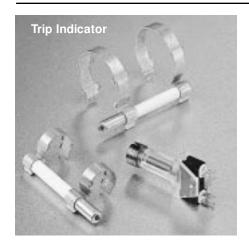
Trip-indicator fuselinks are available for use in parallel with the main fuselinks. They can either be attached to the associated fuselink or mounted separately in panel mounted fuse clips, Part No. CL1. A push-on adaptor and microswitch attachment is available for use with the trip indicator to give the facility of remote indication, reference MAI or MBI.
