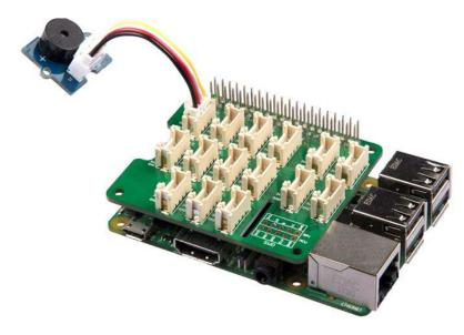
Tap the following command sudo <code>grove\_pwm\_buzzer</code> in the command line interface.
