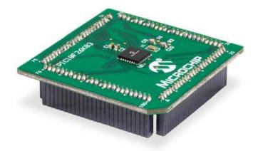
PIC18F26K83 Plug-In Module (Part # MA180037)
