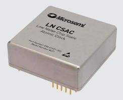
The LN CSAC accepts a 1 PPS input that may be used to synchronize the unit's 1 PPS output to an external reference clock with  $\pm 100$  ns accuracy. The LN CSAC can also use the 1 PPS input to discipline its phase and frequency to within 1 ns and  $1.0 \times 10^{-12}$  respectively.
