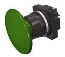
30mm BlackMax, Epoxy Coated Corrosion Resistant Metal Operator, Round Push-Pull Operator Non-Illuminated Mushroom Head Cap Large 2 1/2" (63.5 mm) Plastic, Green 2 Position Maintained, Pull-to-Release UL Listed, CSA Certified NEMA 1,3,3R,4,4X,12,13 & Automotive Standards
