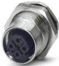
Sensor/actuator flush-type socket, 5-pos., M12 SPEEDCON, B-coded, rear/screw mounting with Pg9 thread, with straight solder connection
