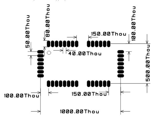
A PCB with two or more layers and with a solid ground plane in one of the inner- or bottom layer(s) is recommended. All GND-pins of the module shall be connected to this ground plane with vias with shortest possible routing, one via per GND-pin.
