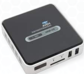
Image Measurement Box Features built-in measurement software with image/video capturing capabilities
