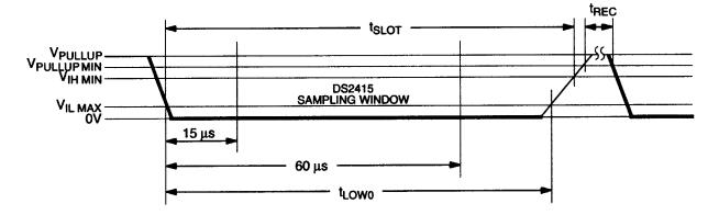
$$60\mu s \leq t_{LOW0} \leq t_{SLOT} \leq 120\mu s \\ 1\mu s \leq t_{REC} < \infty$$
