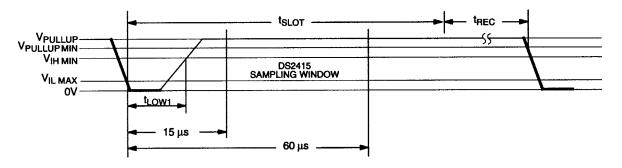
$\begin{aligned} &60\mu s \leq t_{SLOT} < 120\mu s \\ &1\mu s \leq t_{LOW1} < 15\mu s \\ &1\mu s \leq t_{REC} < \infty \end{aligned}$
