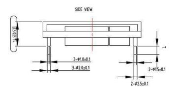
UNIT: mm (inch) L=4.60mm TOLERANCE: X.X mm±0.5mm [X.XX in.± 0.02in.] X.XX mm±0.25mm[X.XXX in.±0.01in.]
