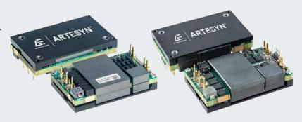
Advanced Energy's Artesyn BDQ1300 & BCQ1300 series quarter-brick are isolated DC-DC converters that produce a single 12V nominal output. Rated at 1300 watts, these converters can deliver up to 107 amps output current and has no minimum load requirement.
