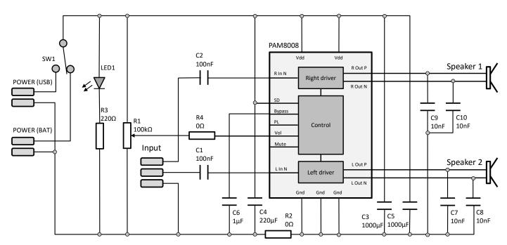
The 3W amplifier uses a PAM8008 amplifier IC, this delivers 3W across the two channels and contains a number of features to make the circuit simple and compact. The device automatically reduces the volume to prevent distortion, has an internal digital volume control and offers over temperature and short circuit protection.
