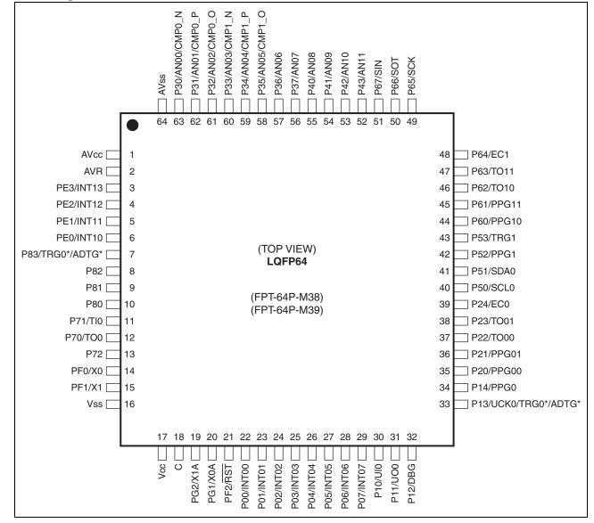
\*: TRG0 and ADTG can be mapped to either P13 or P83 by using the SYSC register.
