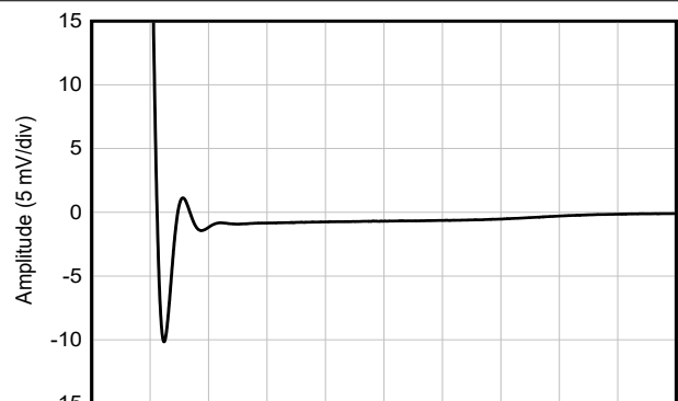
Figure 6-26. Small-Signal Step Response, G = 1
