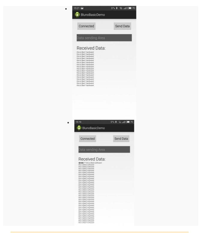
Bee2 <==> Hardware Serial Port; Bee1 <==> Software Serial Port
