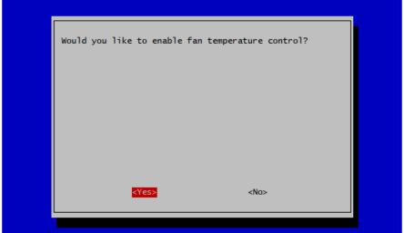
And make sure you put down GPIO pin 4 for the fan
