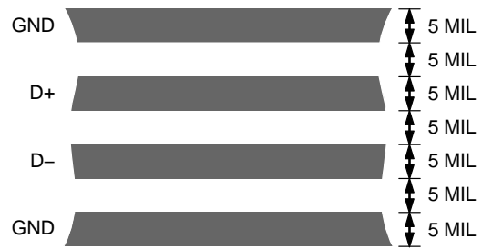
Figure 22. Typical Arrangement of Signal Tracks
