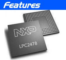
The NXP LPC2478 ARM7TDMI-S based microcontroller runs the open source uEZ<sup>®</sup> + FreeRTOS software platform. The LPC2478 has 512KB of internal Flash memory, 96KB of internal SRAM, a 10/100 Ethernet Media Access Controller (MAC), a USB full speed device/host/OTG controller, four UARTs, two CAN channels and a collection of serial communications interfaces. The uEZGUI board also includes 8MB of external SDRAM and 8MB of external NOR Flash.
