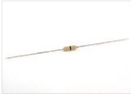
A zerohm jumper looks like a resistor with one black stripe.
