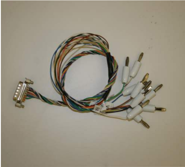
Figure 49. 15-Pin, Twisted Wire Cable to Banana Jacks
