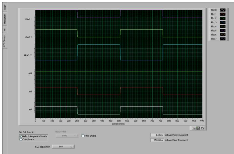
Figure 31. Example of Internal Test Signals Viewed on the ECG Display Tab
