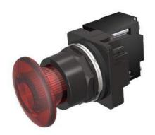
30mm BlackMax, Epoxy Coated Corrosion Resistant Complete Metal Unit Illuminated Push-Pull Operator Transformer type, 120V AC Incandescent Lamp Mushroom Head Cap Small 1 3/4" (44.5 mm) Plastic, Red 2 Position Maintained, Pull-to-Release UL Listed, CSA Certified NEMA 1,3,3R,4,4X,12,13 & Automotive Standards
