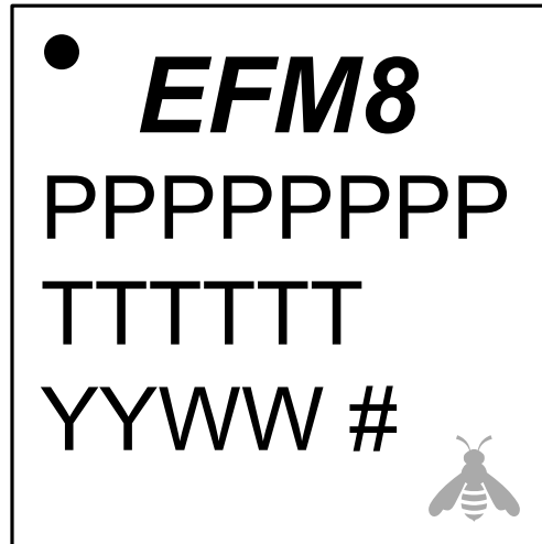
Figure 9.3. QFN32 Package Marking
