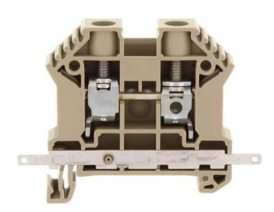
Feed-through terminal, Screw connection, Mounting type: Mounting rail TS 35/7.5, Rated cross-section: 16 mm², Width: 10 mm, Colour: Beige
