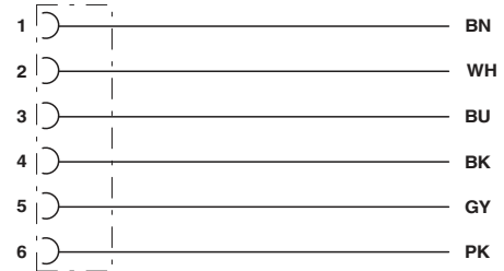
Contact assignment of M8 socket
