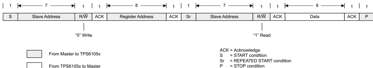
Figure 34. Read Data Transfer Format In F/S-Mode
