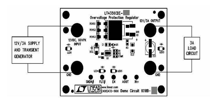
Figure 1: Proper Measurement Equipment Setup
