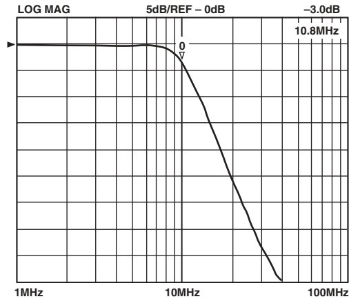
TPC 21. Rx LPF Frequency Response, Low f_c Nominal Tuning Targets
