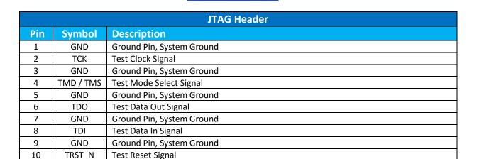
The JTAG header is used in the factory to program the bootloader into the BCM2835 SoC. It can also be used to connect to a compatible JTAG debugger, however should only be utilised by Advanced users who know what they are doing. This header makes for good mechanical support when adding a Daughter Board onto the Armadillo-70T, if nothing else.
