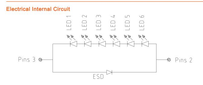
Pins 1: Substrate potential, isolated from Cathode and Anode Pins 2: Anode Pins 3: Cathode
