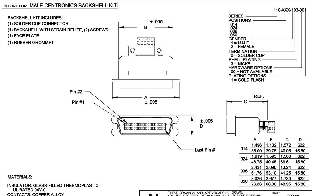
DIELECTRIC WITHSTANDING VOLTAGE: AC 1200 R.M.S. INSULATION RESISTANCE: 1000 mohms MINIMUM AT 500V DC CONTACT RESISTANCE: 30 mOHMS MAXIMUM OPERATING TEMPERATURE: -55°C TO +125°C
