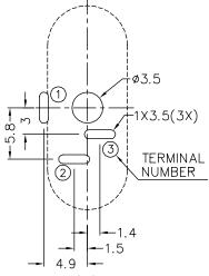
Recommended PCB Layout Top View
