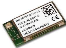
Every BT730 series Bluetooth® module from Laird Technologies is designed to add robust, long-range Bluetooth data connectivity to any device. Based on the market-leading Cambridge Silicon Radio (CSR) BC04 chipset, BT730 modules provide exceptionally low power consumption with outstanding Class 1 range via 18 dBm of transmit power. A broad range of Bluetooth profiles such as Serial Port Profile (SPP) and other vital features make BT730 modules superior to other Bluetooth modules.
