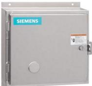
Non-reversing NEMA contactor, Size 0, Three phase full voltage, Contactor amp rating 18A, 3 wire (NO aux included), 220-240/440-480VAC 60Hz coil, Noncombination type, Encl NEMA type 4X 304 S-Steel, Water/dust tight noncorrosive, Extra-wide enclosure
