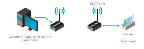
One SNAP Link Adaptor controls multiple SNAP Link serial wireless adapters (either RS-232 or RS-485/422).
