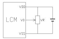
V<sub>DD-</sub>V<sub>0</sub>: LCD Driving voltage VR: 10k~20k
