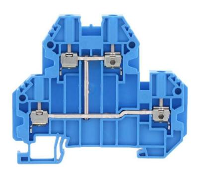
Double-level terminal, Screw connection, Mounting type: Mounting rail TS 35/7.5, Rated cross-section: 2.5 mm², Width: 5.1 mm, Colour: Blue
