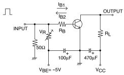
IC=10I<sub>B1</sub>= -10I<sub>B2</sub>=500mA, V<sub>CC</sub>=25V (For PNP, the polarity is reversed.)
