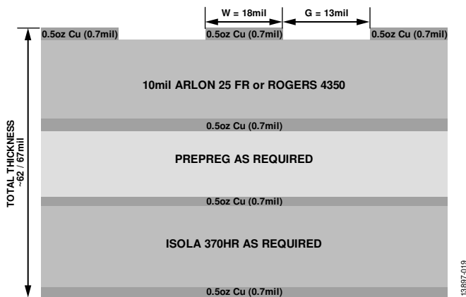
Figure 94. Evaluation Board Cross Sectional View
