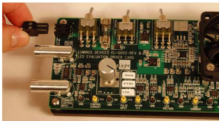
Figure 7: Power supply cable to driver card
